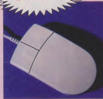
The ST may be a great computer but the mouse that comes with it simply is not up to scratch. The *ST Review* mouse is a major enhancement because it uses micro-switches for the buttons, making it much lighter and easier to click. Our mouse also has a much higher resolution - 280 dots per inch which means you need far less desk space and get much finer control.
